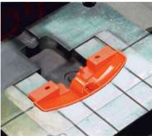
Injection mould - Impact 200 end piece
